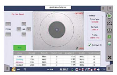
MT1000A screen displays details of the fiber tip core, cladding, adhesive and contact, with automatic Pass/Fail result judgement.
