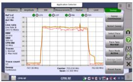
Activating a second trace with Max Hold simplifies identification of intermittent interferers.
