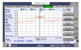
Reducing the span bandwidth gives a detailed view of the interferer signal spectrum, in this case an FM signal. Knowledge of the nature of the interferer gives invaluable information to enable the source to be located.
