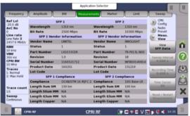
It is essential that the SFP in the tester matches the requirements of the CPRI link under test. Typically the SFP capability data is hard to read from the manufacturer's label. MT1000A conveniently displays the full configuration of each SFP inserted into ports 1 and 2.
