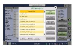
Select Radio type to send the correct commands to initiate a LTE waveform transmission.
