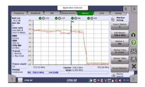
Marker to center frequency positions the interferer to be examined in the center of the display, allowing the user to zoom into the signal for detailed examination.
